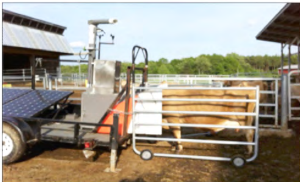
Figure 2. The GreenFeed system being used at the UNH Organic Dairy Research Farm for methane measurements.
